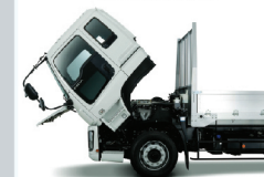
Electronic Cab tilt system
