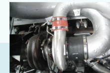
Intercooled-turbocharger maximizes low speed performance and acceleration
