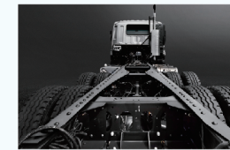
320 mm double channel, strongest-in-class frame
